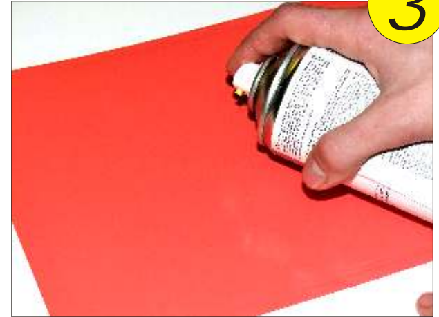
After cutting, remove flock material and apply Spray Mount to the back of the flock material
