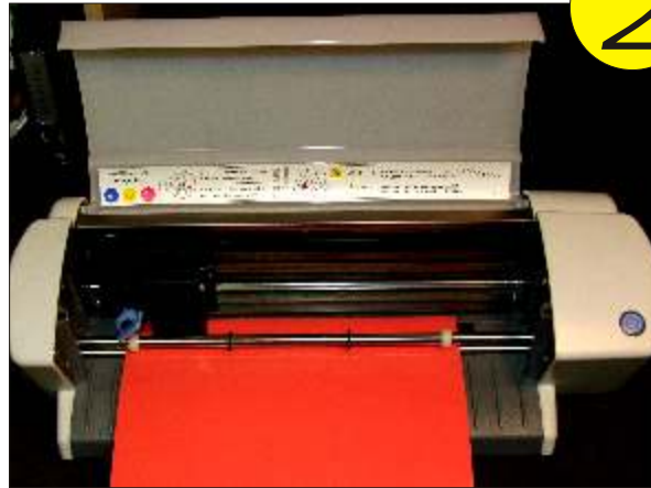
Feed flock material into the Craft Robo, matt side up. Change blade cap to yellow.
